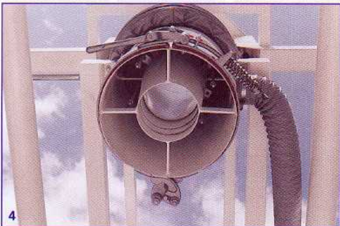
Filling head with telescopic inner pipe. Manual bag spout clamping by one-hand bag clamp
