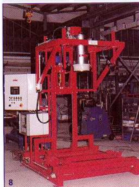
EMDE filling station type BFR 4000E. Weigher can be calibrated, printer for reporting.
