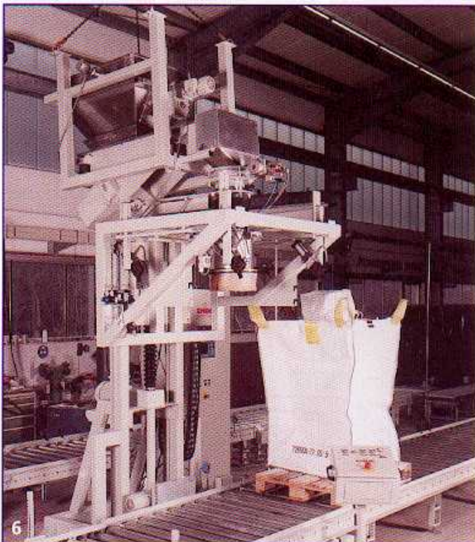
EMDE combination filling station for filling big-bags and boxes. Interchangeable filling pipe and additional precision weigher for small packages. Metering by EMDE-vibrating feeder, roller conveyor for pallet transport.
