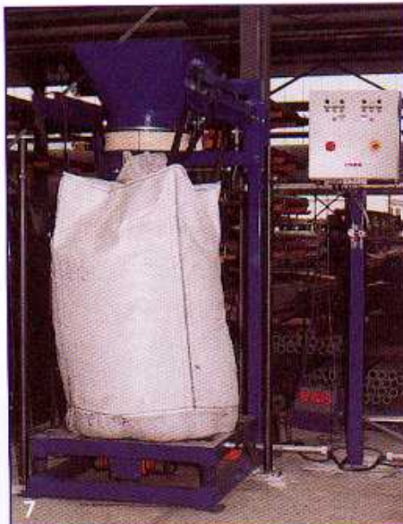
Volumetric Filling with vibration system. EMDE big-bag filling station type BFV 1500
