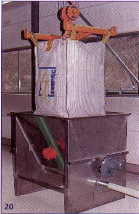
20. EMDE big-bag discharger type BE 1000 with integrated loosening activator and connection for a flexible screw conveyor EMDE-LIFT.
