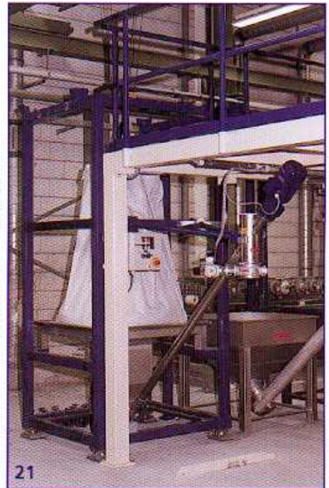
21. EMDE big-bag discharger type BE 1000 S with weighing system for precise discharge dosing. The weigher has a resolution of 100g over a 1500 kg weighing range. Larger batches are also possible owing to the special software with remainder memory.
